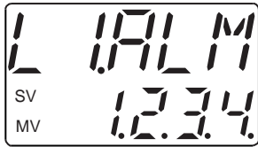
Alarms 1 to 4 are all activated
