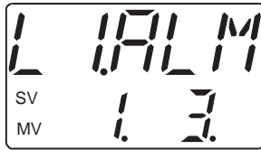
Alarm 1 and 3 are activated
